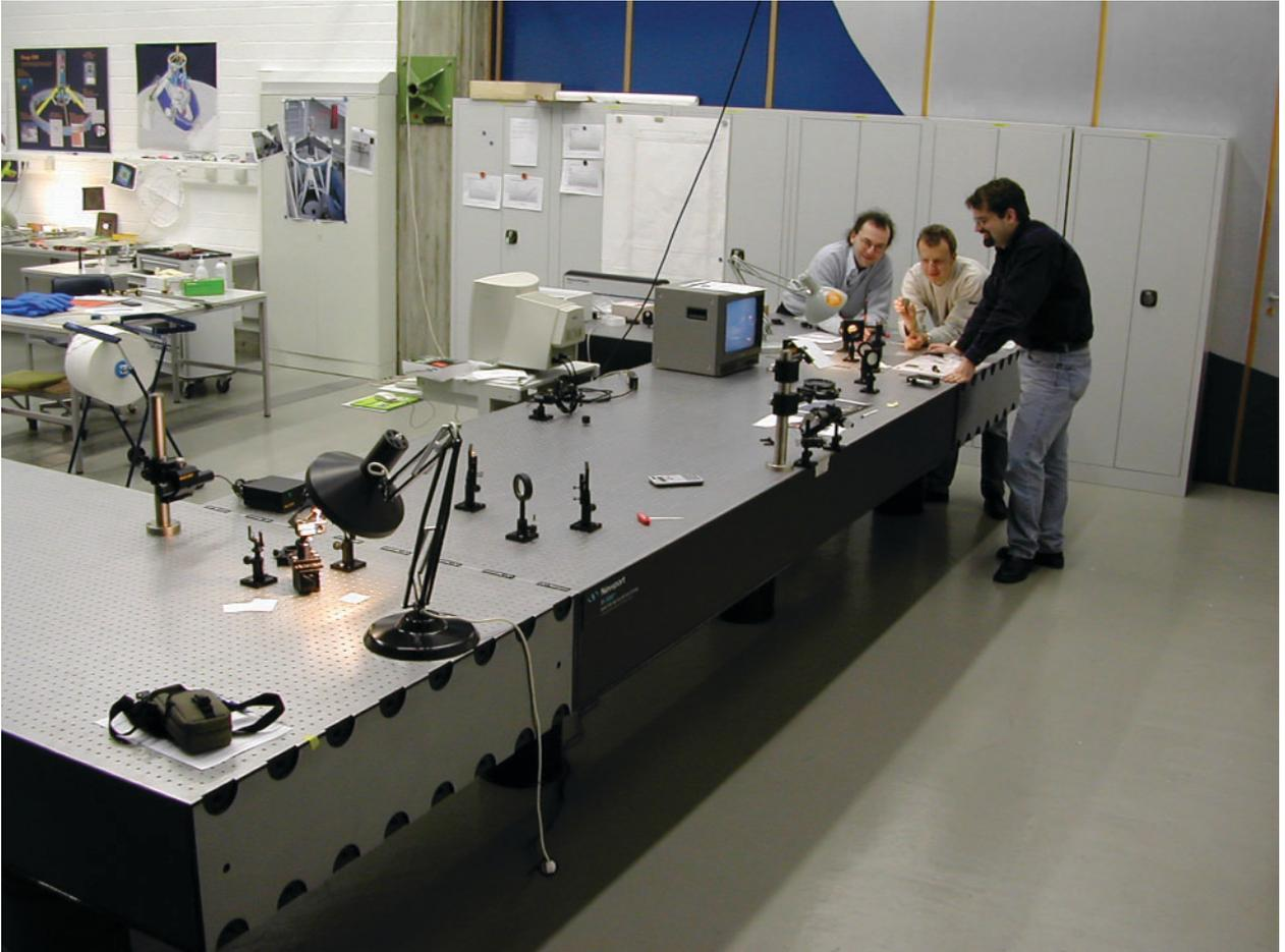
**Fig. IV.5:** The optical bench for testing the folded light path in the planned LINC instrument.
