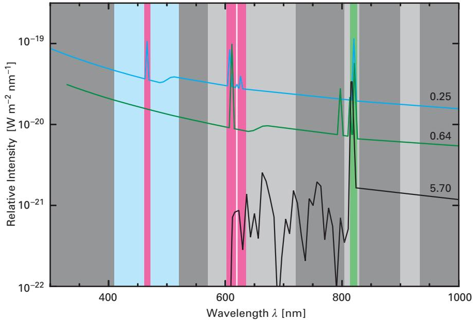
**Fig. III.34:** The CADIS observation method. The pass band of the Fabry-Perot filter for the Lyman- $\alpha$ -line at  $z = 5.7$  is plotted in green, those of the veto-filters in red and light blue. Three spectra with redshifts  $z = 0.25$ ,  $0.64$ , and  $5.7$  are represented schematically.
