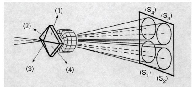
**Fig. IV.2:** The pyramid splits the beam focused onto its tip into four. A zoom lens then creates four pupil images on the detector.
