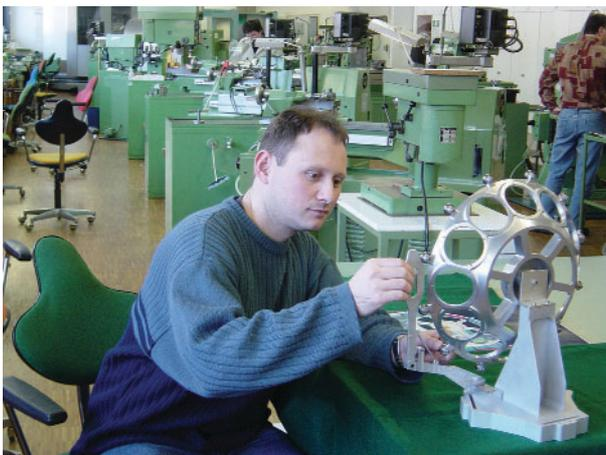
**Fig. IV.10:** Prototype of a filter wheel for NIRSPEC. The wheel was designed computer-aided at the Institute and manufactured online with highest precision using a numerically controlled milling machine.
