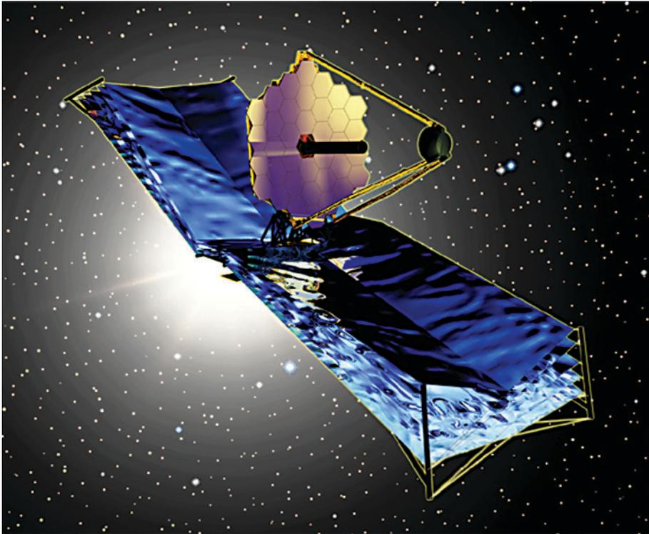
**Fig. I.6:** Possible structure of the NGST, with the large primary mirror and the characteristic solar screen. (Image: TRW)
