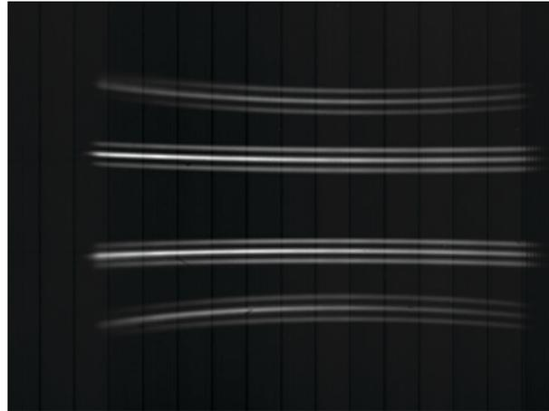
**Fig. II.20:** Channel layout on the detector in the spectroscopic mode with the prism (left) or the grism (right). Two interferometric (middle) and two photometric (outside) channels are to
